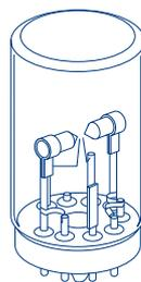
Eliminate degradation of photosensitive samples. A diode array continuously exposes the sample to the entire wavelength range while the Xenon lamp only flashes when acquiring a data point and only exposes the sample to a very narrow wavelength range for each data point.
