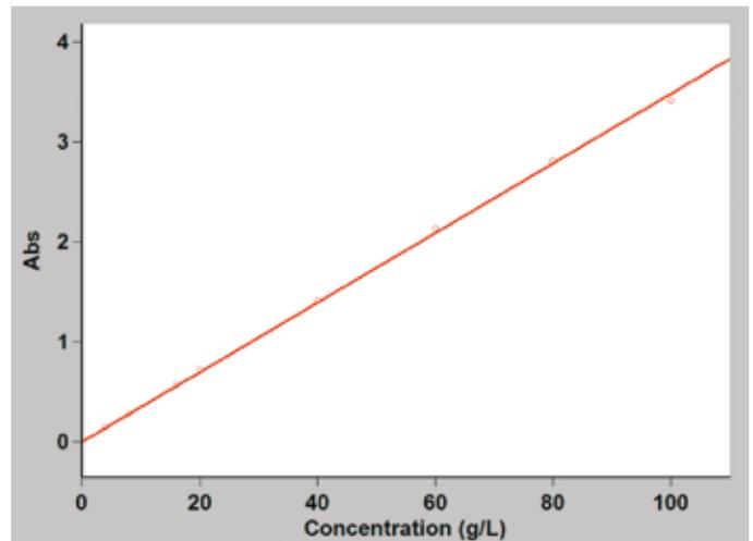
The Varian Cary 50's excellent linearity makes it ideal for measuring samples up to 3.5 Abs accurately and with confidence.
