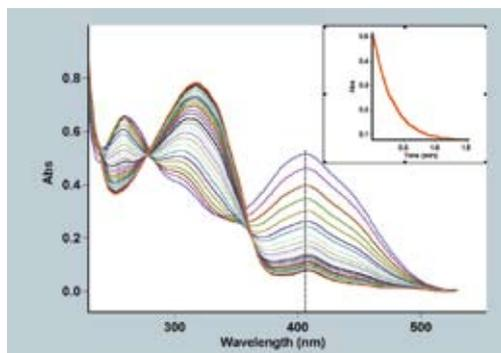
The Cary 50's extremely fast scan speed means that you can repetitively scan your kinetics sample many times during the reaction. Shown are 30 scans collected over 1 minute. The insert shows the kinetics curve at 410 nm.
