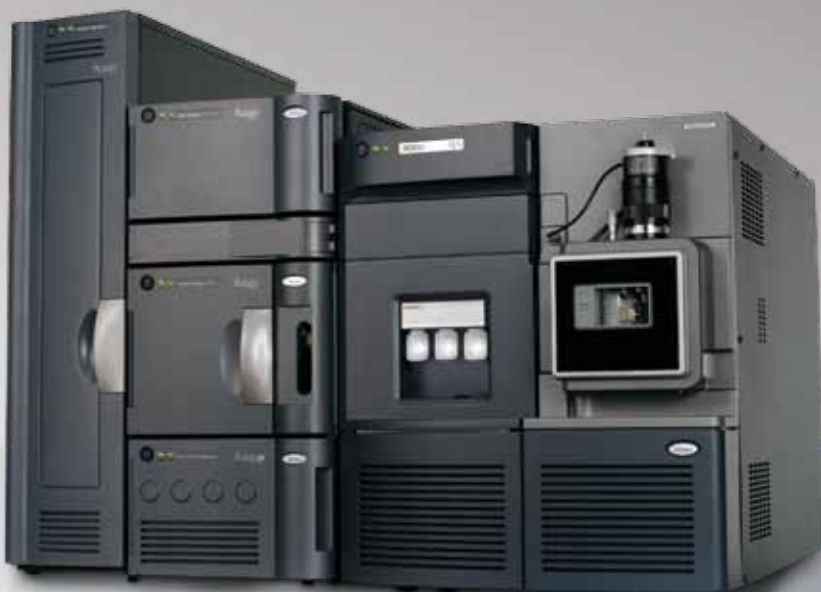
ACQUITY UPLC I-Class System with Xevo TQ-S.
